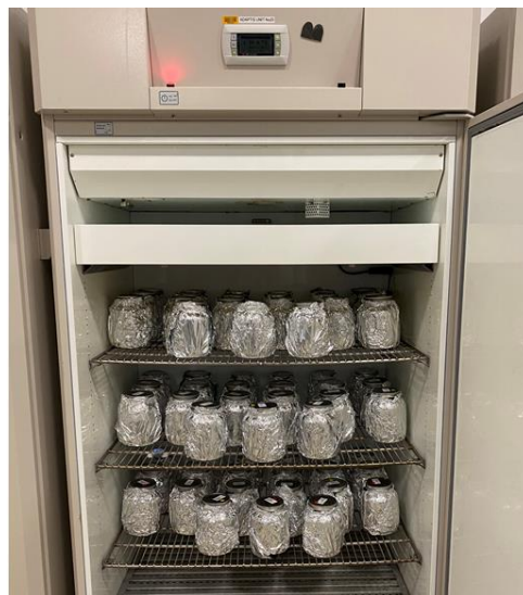
Figure 15: Sample jars setup at 20 °C in a constant temperature chamber at CSU, Wagga Wagga.
