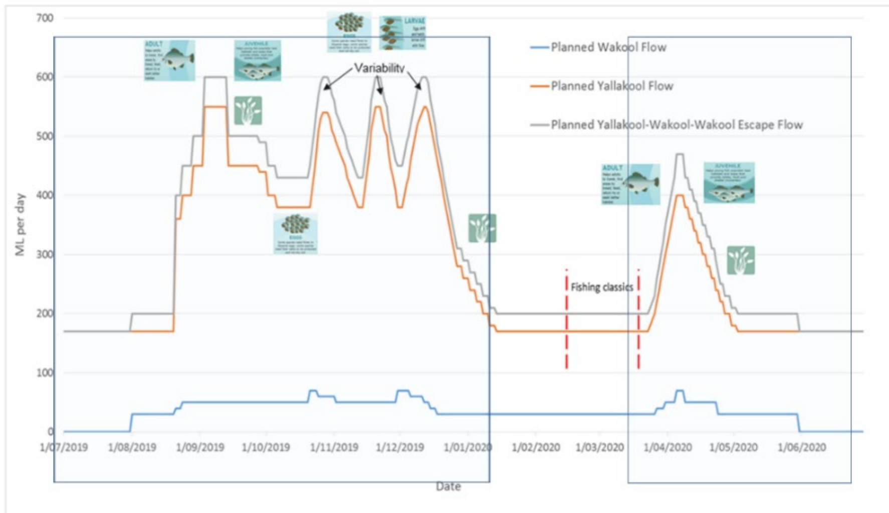
Figure 2.1. Annual hydrograph planned for Yallakool-Wakool at start of 2019-20 action. Shaded area shows period of potential use of CEW. Operational base flows are usually around 170 ML/day except in winter when they are zero unless provided via unregulated flows. (Source: CEWO 2019)
