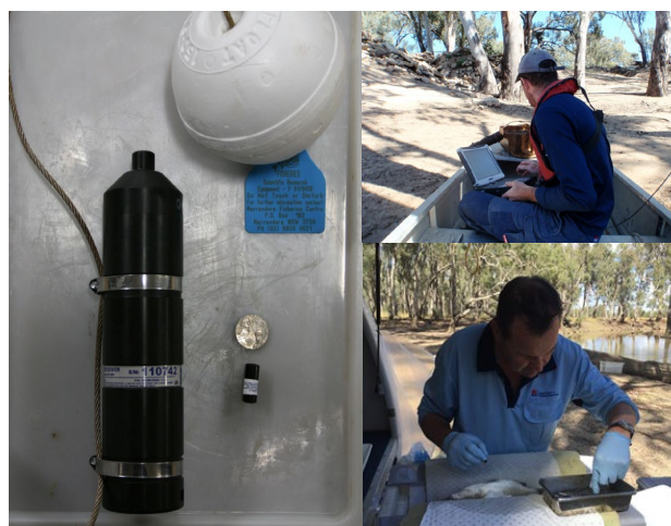
Figure 8.3 Clockwise from left: An acoustic receiver ready for deployment and an acoustic tag for scale, downloading information from tagged fish passing an acoustic receiver and, an anaesthetised silver perch undergoing surgical implantation of an acoustic tag.
