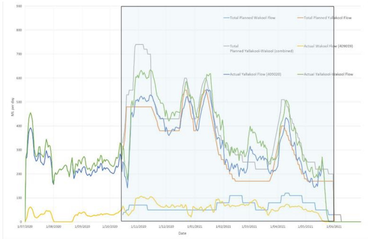
Figure 2.4 Annual hydrograph for Yallakool-Wakool at end of 2020-21 action, showing the change made to the planned flows due to greater water availability in the Murray system. Operational flows were provided from October – June following initial unregulated flows wetting up in the system. Shaded area shows period of CEW use. (Source: CEWO 2021).
