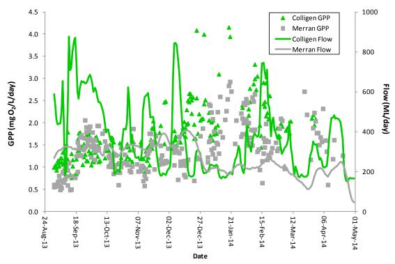
**Figure 53.** Gross Primary Production (GPP) rates and stream discharge for Colligen and Little Merran Creeks from September 2013 through April 2014. The paucity of data from Colligen Creek from mid-February onwards is due to problems with the DO sondes.
