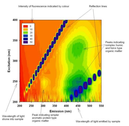
Figure 47. Sample excitation emission contour plot indicating key features of the data. (Watts et al. 2013a)
