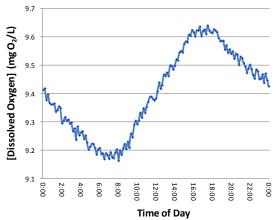
**Figure 51.** Typical Dissolved Oxygen Concentration Profile over a 24 hour period. This unsmoothed data was from Yallakool Creek on the 6<sup>th</sup> October, 2013. The signal may appear noisy but is actually very stable given the small diurnal change in concentration.
