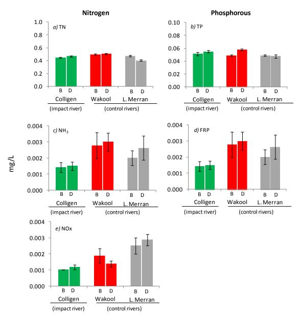
**Figure 46.** Colligen-Niemur continuation flow: BACI comparison of nutrient concentrations between treatment and control rivers for the Colligen-Niemur continuation flow – the first bar of each pair is before (B) the watering action, the second is after (A) the watering action.
