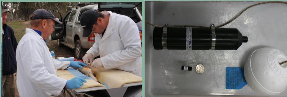
Photos: left, Surgery to insert tags into fish. right; A VR2W acoustic receiver rigged for deployment next to a V13-1x A69 acoustic tag.
