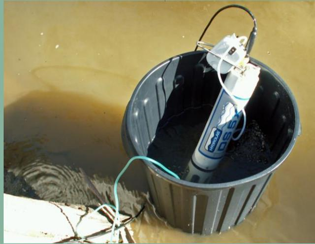
Photo: Dissolved oxygen logger being calibrated in the field
