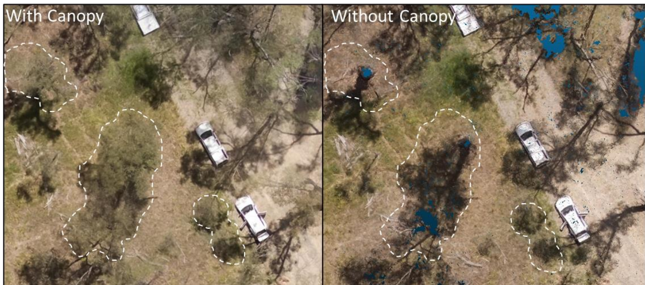
Figure 4. Left - An aerial photo with ground cover obscured by tree canopy. Right - raster image generated after the canopy has been removed. Note: some shadows remain after canopy removal (dark patches in right image), and some holes (blue areas) occur where groundcover vegetation cannot be assessed.
