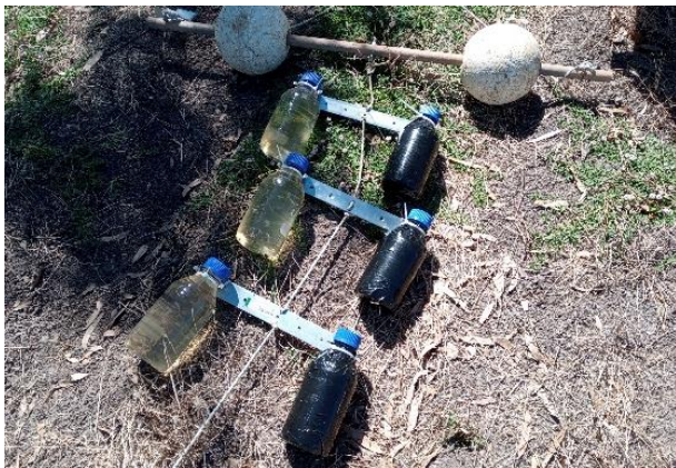
Figure 6. Left - Incubation bottles used for measuring primary productivity. Right - Experiment in Colligen Creek (Photos: Andre Siebers).
