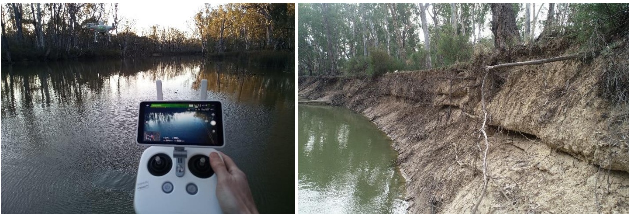
Figure 6: Left, Drone in flight. Right, A section of riverbank downstream of Stevens Weir highlighting the notch that aligns with the height where discharge in the range of 2300 to 2800 ML/day occurs.
