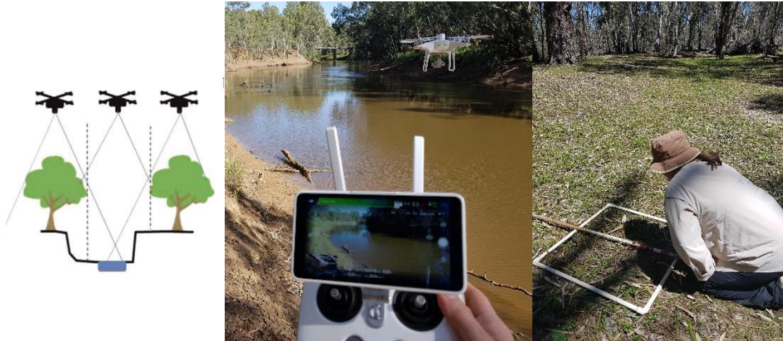
Figure 3: Left - A drone will be flown above the forest canopy to collect colour and multispectral imagery, and three-dimensional elevation data to assess ground vegetation condition. (Photo: Streamology. Right - Ground surveys of vegetation in Werai Forest will be conducted simultaneously with drone flights to ground-truth the drone data (Photo: Robyn Watts)
