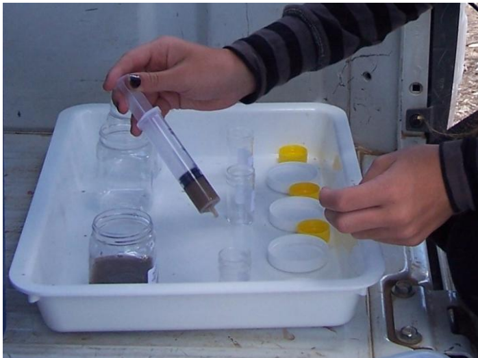
Figure 32. A 20 mL sample of the biofilm residue is collected for the assessment of taxonomic composition
