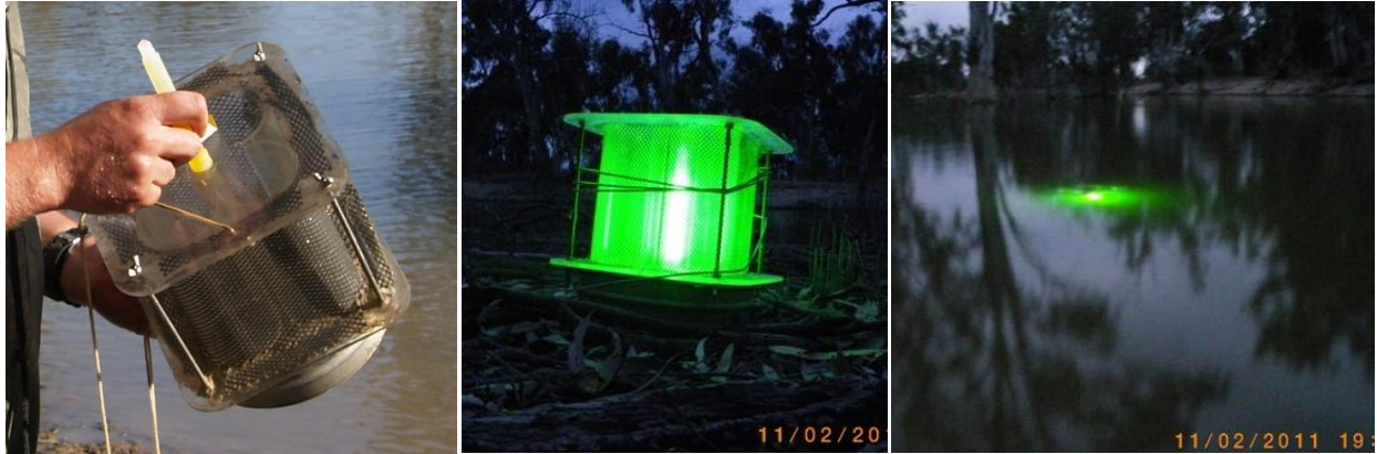
Figure 87. Photos of light traps used to sample larval fish, showing bioluminescent light stick in the centre of the trap
