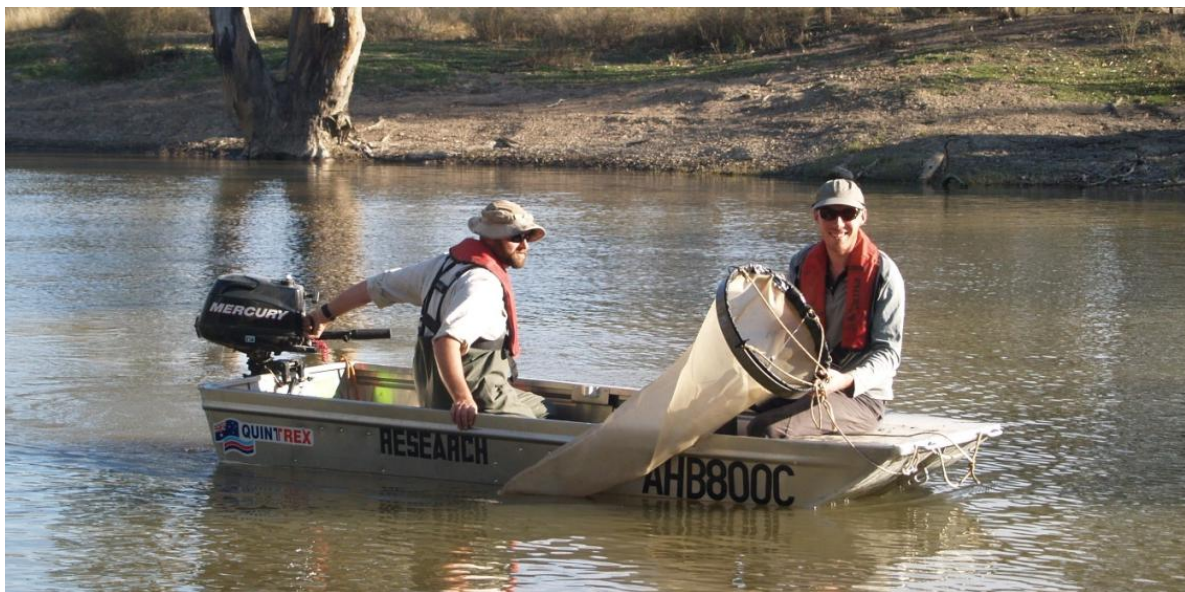
Figure 88. Drift net used to undertake boat trawls for larval fish. This sampling method is undertaken after dark.
