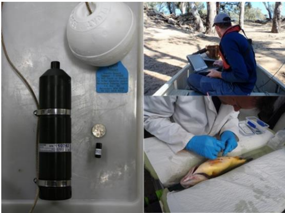
Figure 8.1. Clockwise from left: An acoustic receiver ready for deployment and an acoustic tag for scale, downloading information from tagged fish passing an acoustic receiver and, an anaesthetised golden perch undergoing surgical implantation of an acoustic tag in August 2015.
