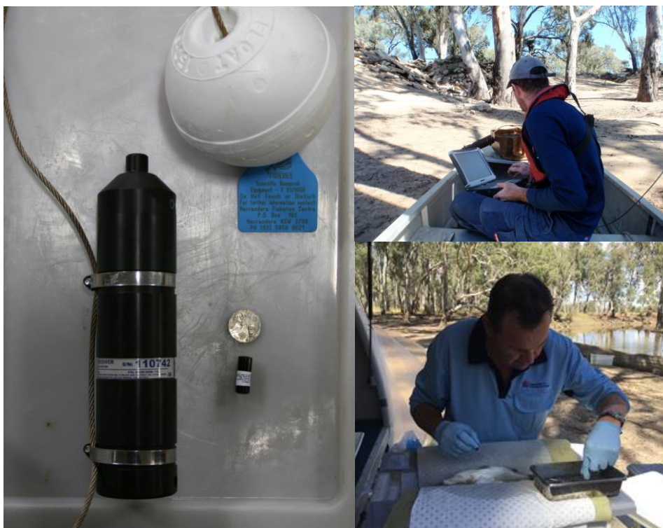
Figure 8.1 Clockwise from left: An acoustic receiver ready for deployment and an acoustic tag for scale, downloading information from tagged fish passing an acoustic receiver and, an anaesthetised silver perch undergoing surgical implantation of an acoustic tag in April 2017.
