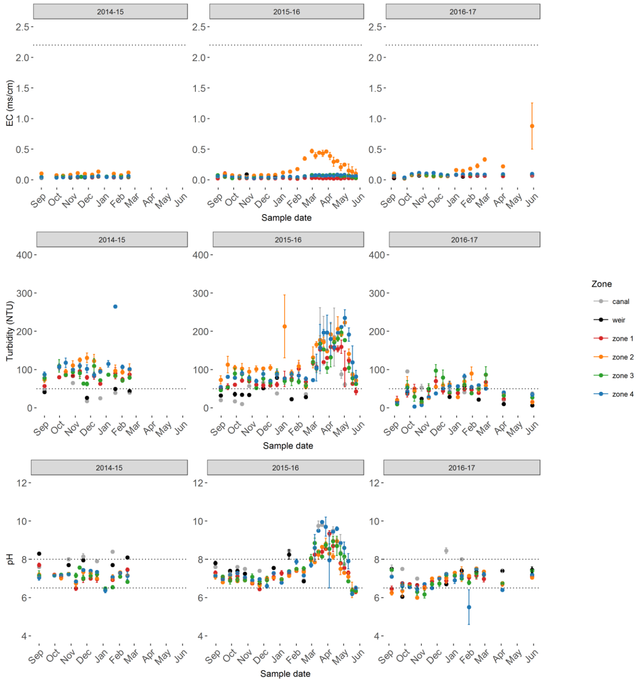
Figure A5 Electrical conductivity, turbidity and pH for LTIM sites and source water over the 2014-15, 2015-16 and 2016-17 sampling seasons.
