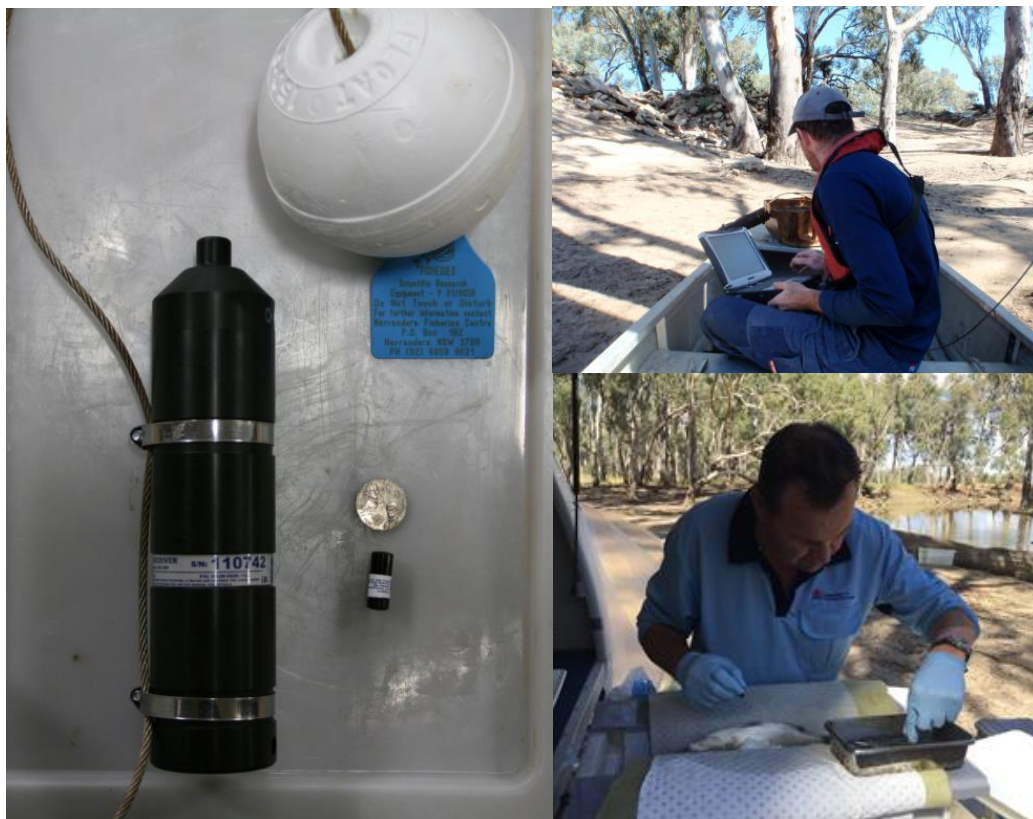
Figure D3 Clockwise from left: An acoustic receiver ready for deployment and an acoustic tag for scale, downloading information from tagged fish passing an acoustic receiver and, an anaesthetised silver perch undergoing surgical implantation of an acoustic tag in April 2017.
