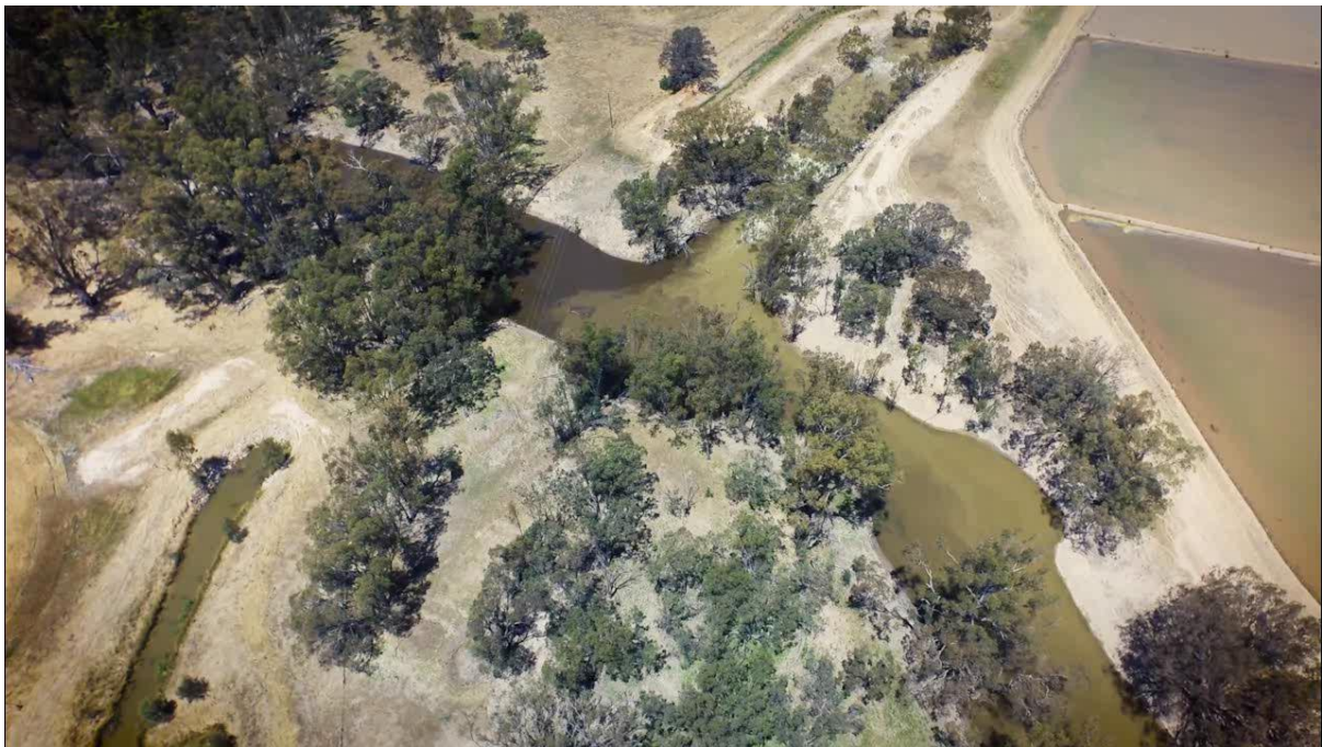
Figure A25 Images showing the release of CEW into the Wakool River at a Flow rate of 500 ML/day. Turbidity differences indicate zones of incomplete mixing where high turbidity water is expected to also have higher dissolved oxygen. Photos: Top, Damian McRae, CEWO; Bottom CEWO.
