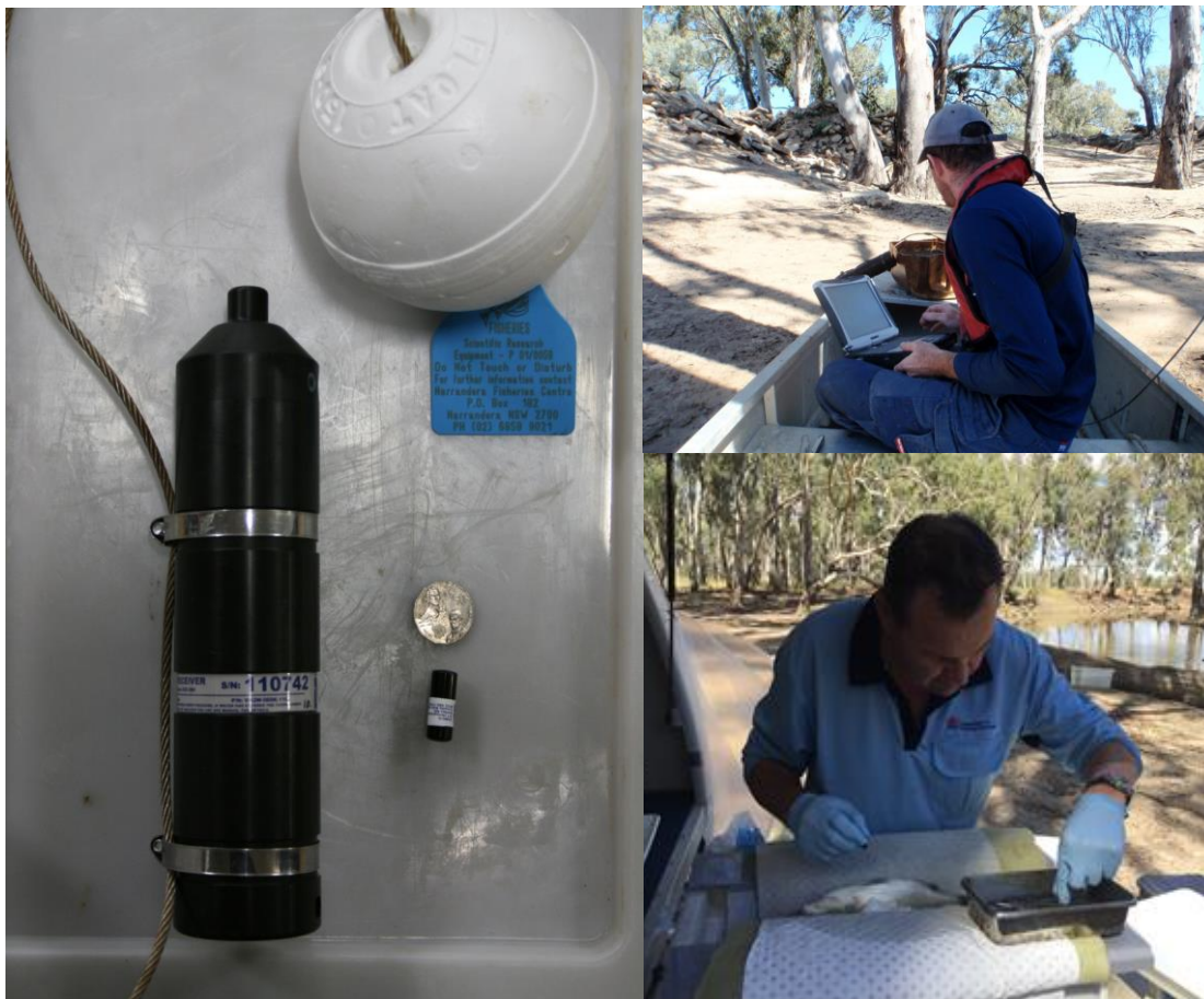
Figure 8.3 Clockwise from left: An acoustic receiver ready for deployment and an acoustic tag for scale, downloading information from tagged fish passing an acoustic receiver and, an anaesthetised silver perch undergoing surgical implantation of an acoustic tag.
